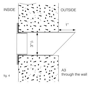
In case of fixed installation, air discharged from rear hose has been extracted from the room where the appliance is installed. Check that the room (especially if small) is not "air-tight"; a drop in pressure would cause irregular functioning, which could consequently activate reset switch. Air entering through door and window cracks is normally sufficient. If deemed, necessary leave a door ajar (approx. 1 cm is enough).
